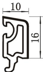
VT88-SY Double glazing bead Unit Weight 0.145 kg/m
